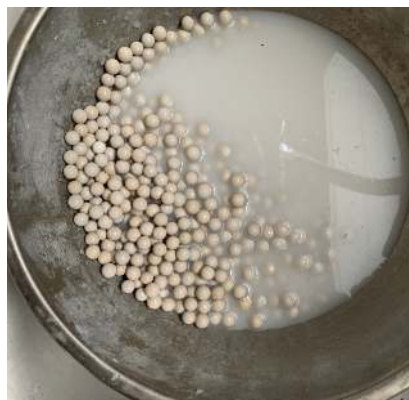
Figure 10: Neutralization media that has been rinsed with clean water
