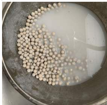
Figure 5: Neutralization media that has been rinsed with clean water
